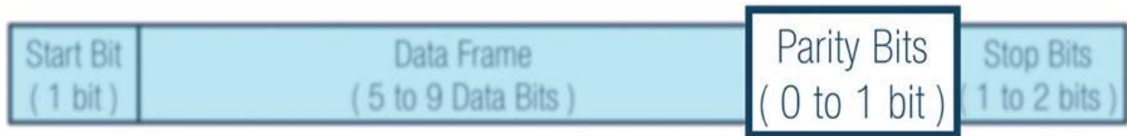
Fig 2.1.6 Check or Parity bit
